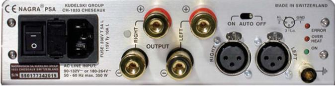
You can configure the PMA to accept balanced or unbalanced inputs, while the PSA is limited to balanced inputs. A switch on both enables or disables the auto-on function, which turns the amp on when it receives a signal and shuts it down after 15 minutes of silence. This is especially helpful when the amps are inaccessable — though they are attractive enough to want them visible.
